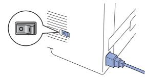
Plug the AC power cord into an AC outlet. Turn the power switch on.
